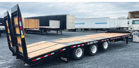
NEW - BWS 22.5 Ton and 30 Ton Air Tilt Tags in Stock. Paver Ramps. Qty-3 22.5 ton Qty-3 30 ton
