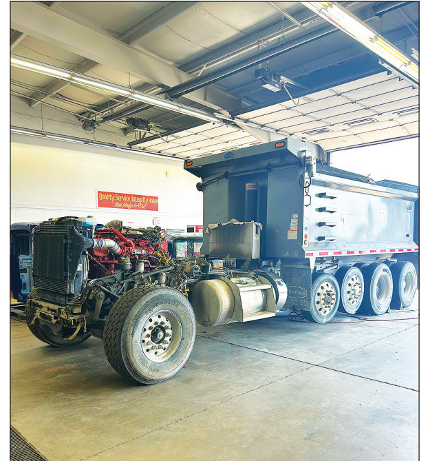
Cabs and bodies are removed and replaced.
