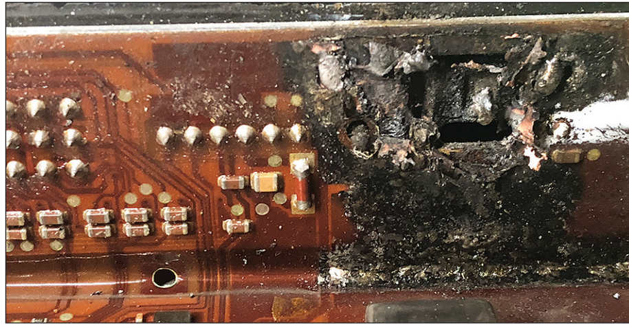
Burned through ground supplies and melted solder indicate that this DDEC got fried through its grounds.
