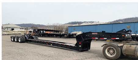
60-TON BEAM Qty 1 - Fontaine Magnitude 60 MBMD, 28' Beam, Modular Connection at Rear.
