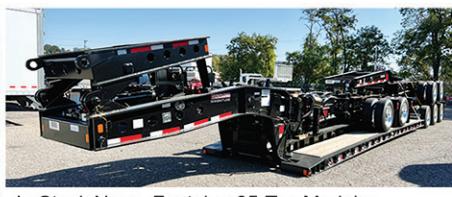
In Stock Now - Fontaine 65-Ton Modular Drop-Side Rail, 28' Well, 60" Axle Spacing, Pony Motor, 70" Hydraulic Flip Box, 2 Axle Jeep, EQ2 Hydraulic Spreader, Intermediate and Rear Flip Axles.
