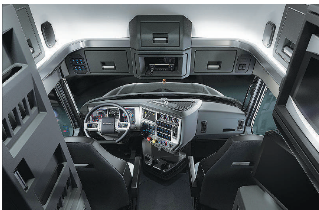
The redesigned dash includes a flat-bottomed steering wheel for easier egress to the driver's seat.
