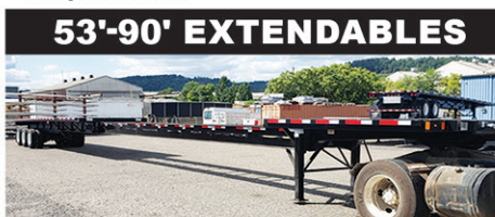
Qty 5 - New Fontaine 53'-90'x102" Xcaliber Extendable Flatbeds, Tri-Axle, Air Ride Sliding Tridem, Cal Legal.
