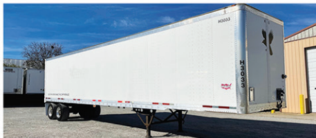
Qty 40 - 42' Wabash-Dry Vans, 42'x96"x12'5", 2- 10' E-Track Rows at 24" & 54" Heights, Tire Inflation System, Aluminum Cross Members in Bay Area. (2011/2012 Sheet & Post, 2014/2016 are HBR).
