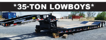
Qty 4 - New Eager Beaver Pavers, 35 GSL-PT Hydraulic Detachable, 35-Ton, 24' Deck, Air Ride. Both Red and Black.
