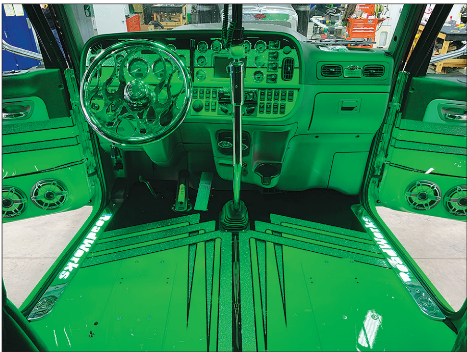
Davis Brother Designs installed the 7200 watt sound system in Night Moves. The sound system features 18 speakers by JL Audio and SounDigital amplifiers.
