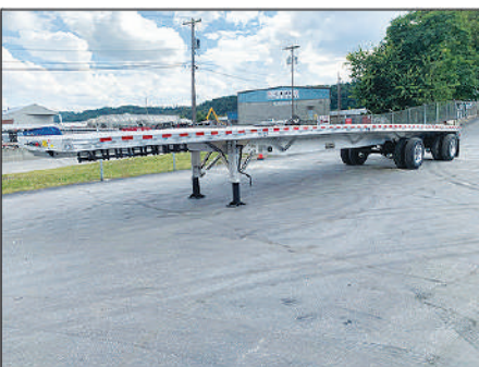
(10) 2025 REITNOUER CK-100 ALUM FLATS 48"x102", Bubba Main Beams, 100,000 Lbs GVWR, Intraax 25K Susp, Coil Pkg, $48,750 Incl FET
