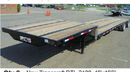
Qty 9 - New Transcraft DTL-2100, 48'x102", Main Deck Length 38', Winch Track on Roadside, Tie Bar on Curb Side.
