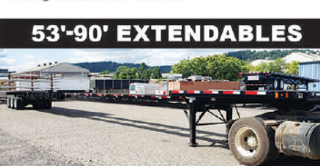
Qty 5 - New Fontaine 53'-90'x102" Xcaliber Extendable Flatbeds, Tri-Axle, Air Ride Sliding Tridem, Cal Legal.
