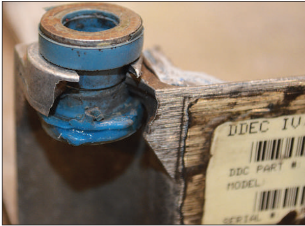
If these mounts were installed, this wouldn't have happened.
