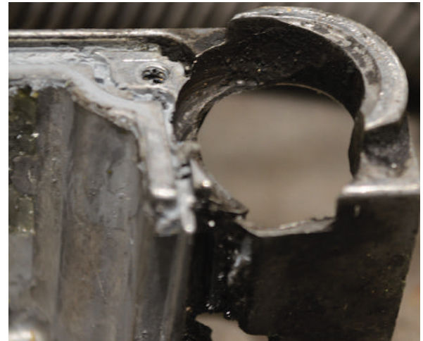
This was the only mounting point that was preventing the ECM from falling off.
