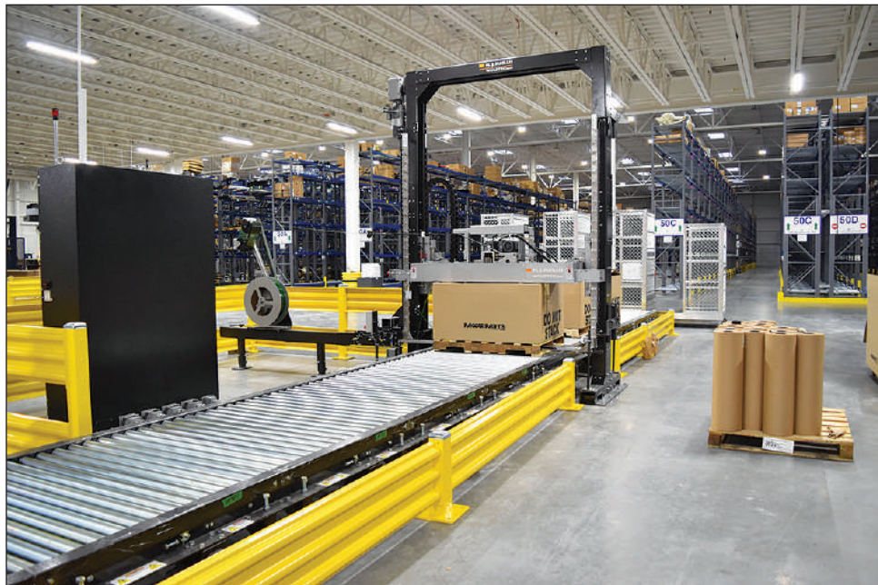
Through state-of-the-art supply chain systems and technology like this pallet-strapping machine and conveyor, equipped with smart sensors, PACCAR Parts fulfills orders from Kenworth and Peterbilt dealers and TRP Stores.
