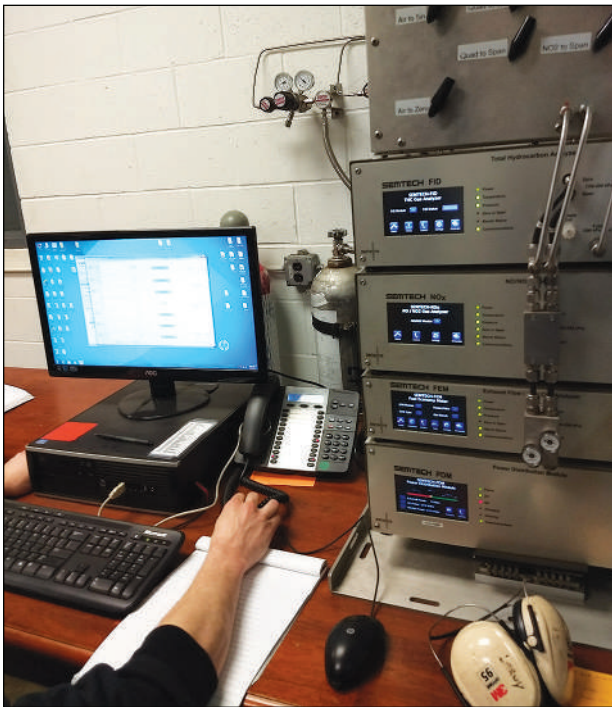
PEMS gas analyser and controller.
