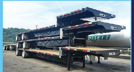
Qty 22 – 2023 Transcraft DTL-2100, 48'x102", Main Deck Length 38', Winch Track on Roadside, Tie Bars on Curb Side, Some with Dump Valves.
