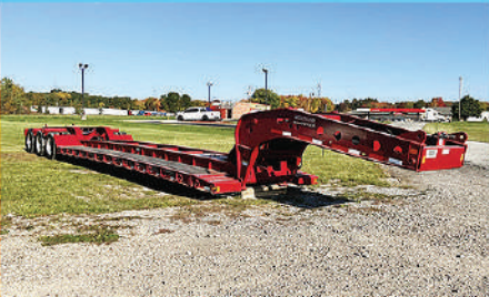
Qty 3 – Fontaine 55HDSR, 53'x102", 55-Ton Capacity, 26' Main Deck Length, 5 Ride Height Positions, Rear Lift Axle, Available in Red & Black.
