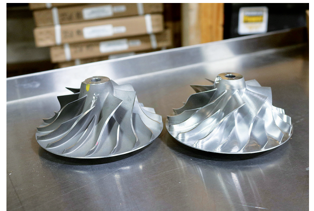
Polished vs. stock turbo wheel
