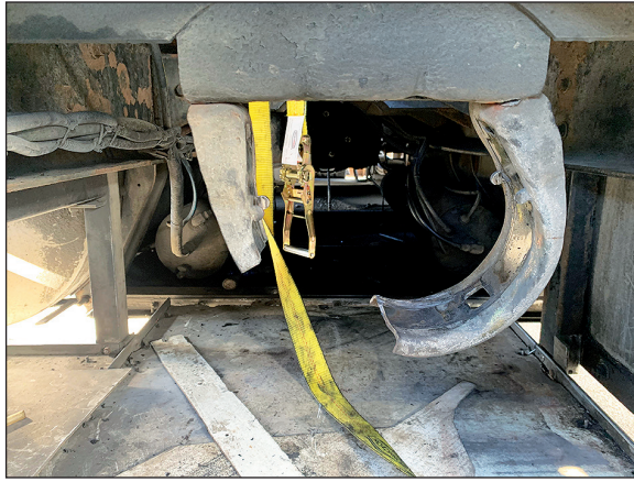
Steve Kron's broken driveshaft bracket.
