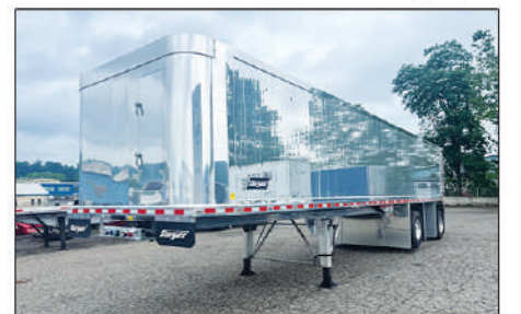
2025 STARGATE 40' ALUMINUM FRAMELESS DUMP 40"x102"x72", Polished Sides, Dual Tailgate, 38 Total Lights per side, 10'2" Spread Frt. Lift Axle, Disk Brakes $99,500
