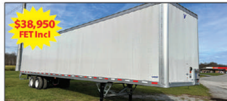
QTY 8 - New Vanguard 53' MaxCube (Sheet and Post) Dry Vans - Air Ride, Swing Doors, Plastic Lined, Logistic Posts on 16" Centers. $38,960 Incl FET
