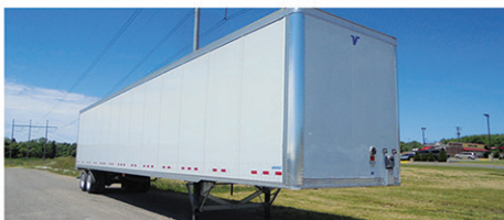
Qty 50 - 2024 Vanguard VXP Plate Vans, 53'x102"x136", 110" Inside Height & Door Opening, Sliding Doors, Air Ride. Also Available w/ Skirts and w/ High Base Rail.
