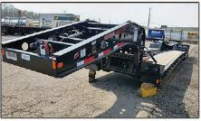
18" Deck Ht, NGB, Air Ride, Rear Axle Lift, Alum Outer Wheels, 275/70R22.5, Strobe Lights, \$108,750
