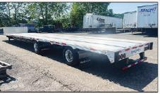
(8) NEW WABASH COMBO 734 LOW PROFILE (10) 2025 FONTANE 55LCC,, 53"x102", 26' Well, DROPS, 53"x102", 36' Rear Deck Ht. Sliding Rear Axle, Cal Legal Alum Outer Wheels, \$59,750 Incl FET
