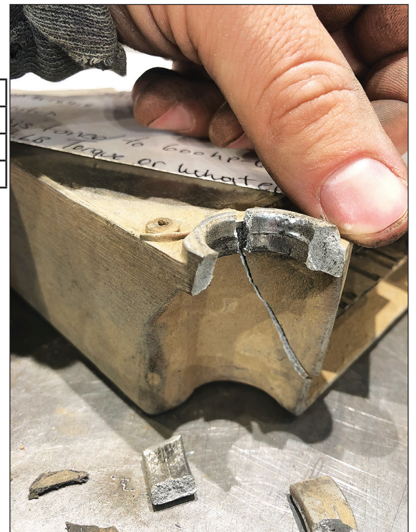
The mounting ears on the corners of the ECM are the easiest to damage.
