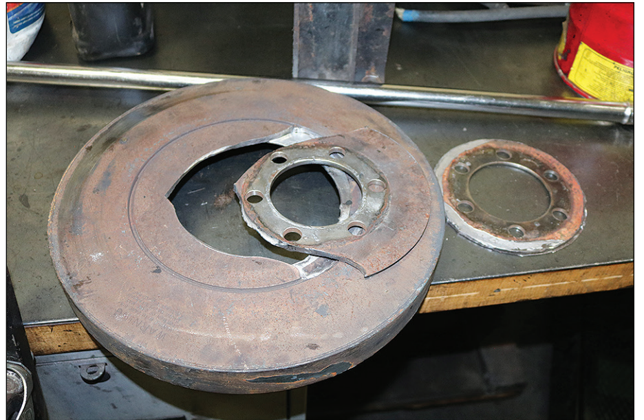
"Broken vibration damper"
