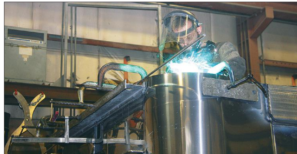
Mike Lacher welding a trailer bulkhead.
