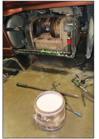
DPF Filter off a truck using Max Mileage FBC
