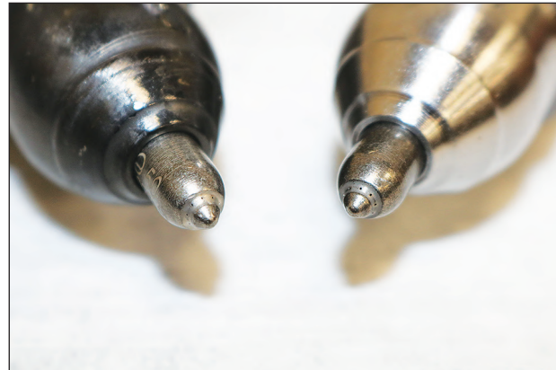
Note the two different sized holes in these injector tips
