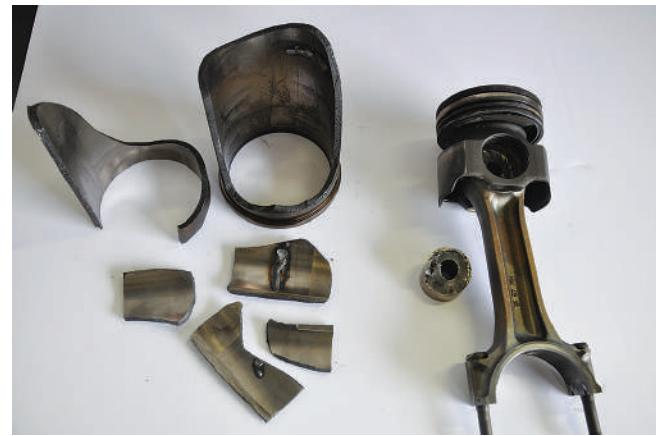
Broken liners and pistons.
