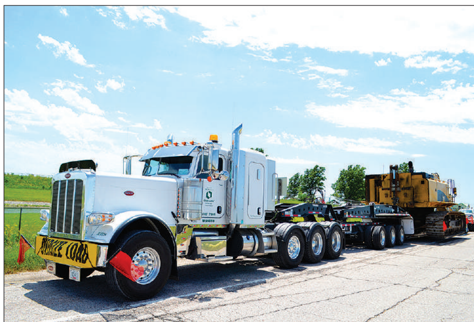
This 2018 Model 389 heavy haul with trailer has a total of 13 axles and totals a 240,000-pound rig. Pulled by a 605 hp Cummins engine.
