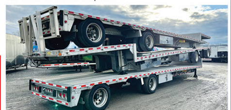
Qty ( 24 ) 2015 / 2016 /2018 Reitnouer Dropmiser 48'x102" Rear Axle Slide , Winch Track both sides, Toolboxes, Disc Brakes
