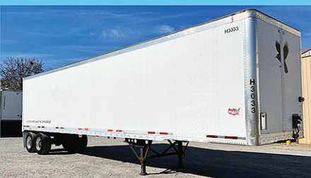
Qty 40 – 42' Wabash-Dry Vans, 42'x96"x12'5", 2- 10' E-Track Rows at 24" & 54" Heights, Tire Inflation System, Aluminum Cross Members in Bay Area. (2011/2012 Sheet & Post, 2014/2016 are HBR).
