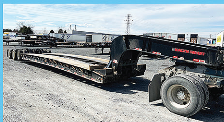
2019 Kalyn Siebert 60-Ton Lowboy, 59'x102", 30' Deck Flip Axle Connections at Rear, Hydraulic Detachable Gooseneck, Dual Hydraulic, Front Lift Axle.
