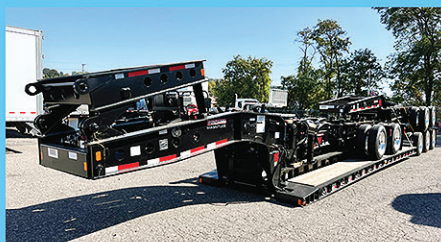
In Stock Now - Fontaine 65-Ton Modular Drop-Side Rail, 28' Well, 60" Axle Spacing, Pony Motor, 70" Hydraulic Flip Box, 2 Axle Jeep, EQ2 Hydraulic Spreader, Intermediate and Rear Flip Axles.
