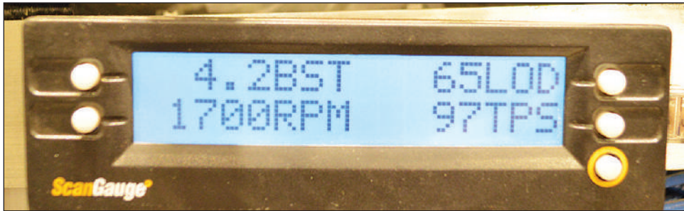
With boost down to 4.2 PSI, this DDEC is holding back at 65 LOD.
