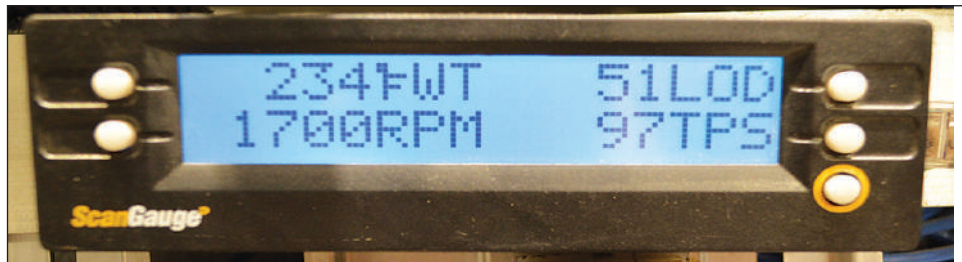
Reading a water temp of 234° F, this DDEC is cutting power to 51 LOD.
