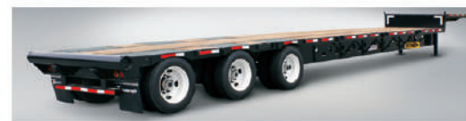
New Transcraft Dropdeck 53'x102 Tridems, Pin Pockets, round pipe at transition, sliding winches
