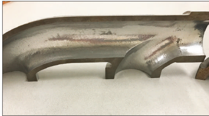
Pittsburgh Power's Full Tilt Manifold. Note: All 45° angles.
