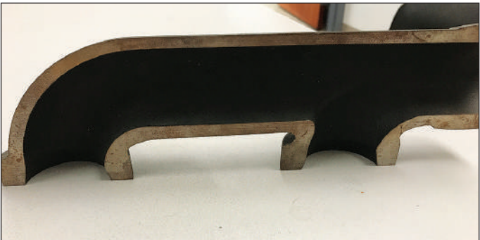
Competitors's stock exhaust manifold. Note: NO 45° angles - all 90° angles.
