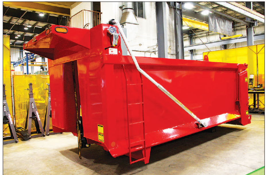
Newly painted Bilbeau body ready to be mounted on a matching Mack Granite tractor.
