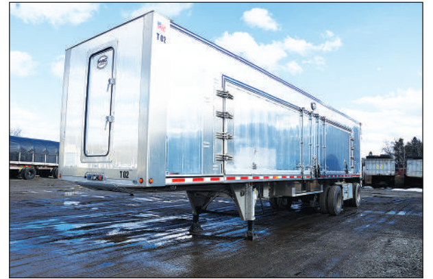
Custom built side loading aluminum dump trailers are the newest addition to the PI&I fleet.
