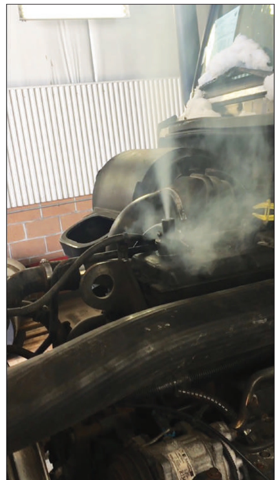
Blow by with a hole in a piston of an N-14 Cummins engine.
