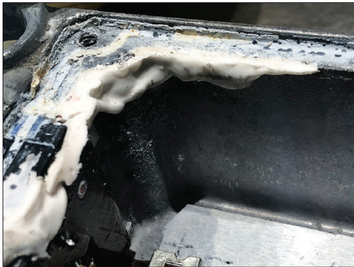
Improper removal and application of sealant during the rebuild caused water damage and allowed the ECM rebuilder to get out of their own warranty.
